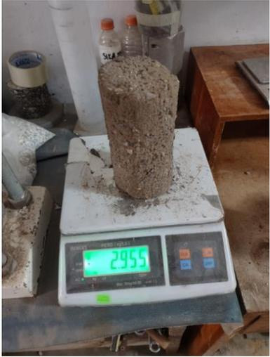
A photograph showing a cylindrical soil sample being weighed on a digital scale. The scale's display is green and shows a reading of 2955. The sample is light-colored and appears to be a soil or sediment. The background shows a laboratory setting with a desk, a pen holder, and some papers. |
