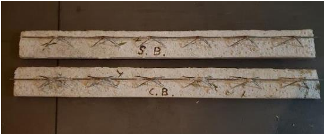
Figura N° 7: Deformación de vigas. Fuente: Use of bamboo of dendrocalamus asper species in premolded concrete beams for deformation analysis (Henrique, 2020)
