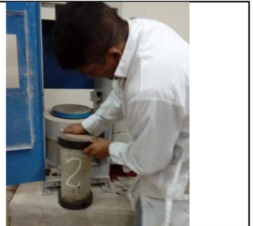
**ENSAYO A LA ROTURA A LA COMPRESION**
