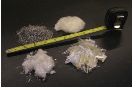
Fig. 5.2.2—Examples of fibers used to control shrinkage cracking.
