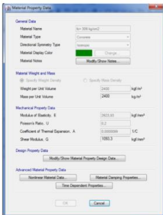
Figura N° 22: Material concreto f_c = 306 \text{ kg/cm}^2
