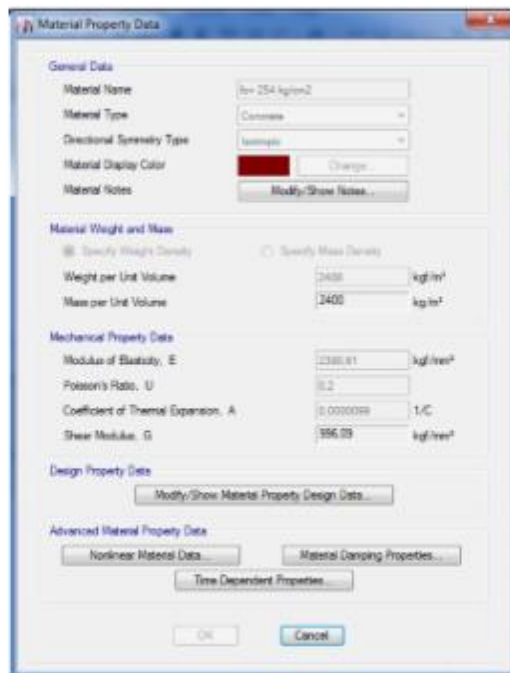
Figura N° 21: Material concreto f_c = 254 \text{ kg/cm}^2
