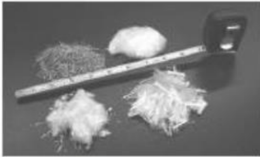
Fig. 2.3—Typical fiber types.
