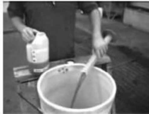
Fig. 2.1—Diluting foam concentrate in water (click on picture to view video).
