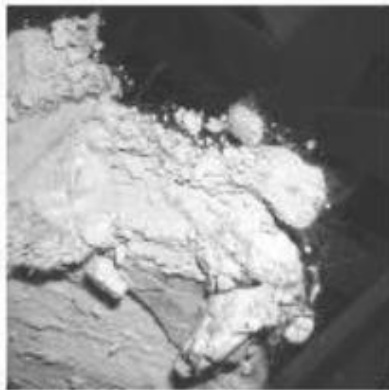
Fig. 2.4—Fibers in cellular concrete.
