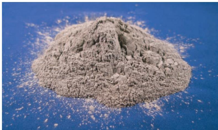
Figura 3: Muestra típica de cemento portland, tomado de Design and Concrete Mixtures, Portland Cement Association.
