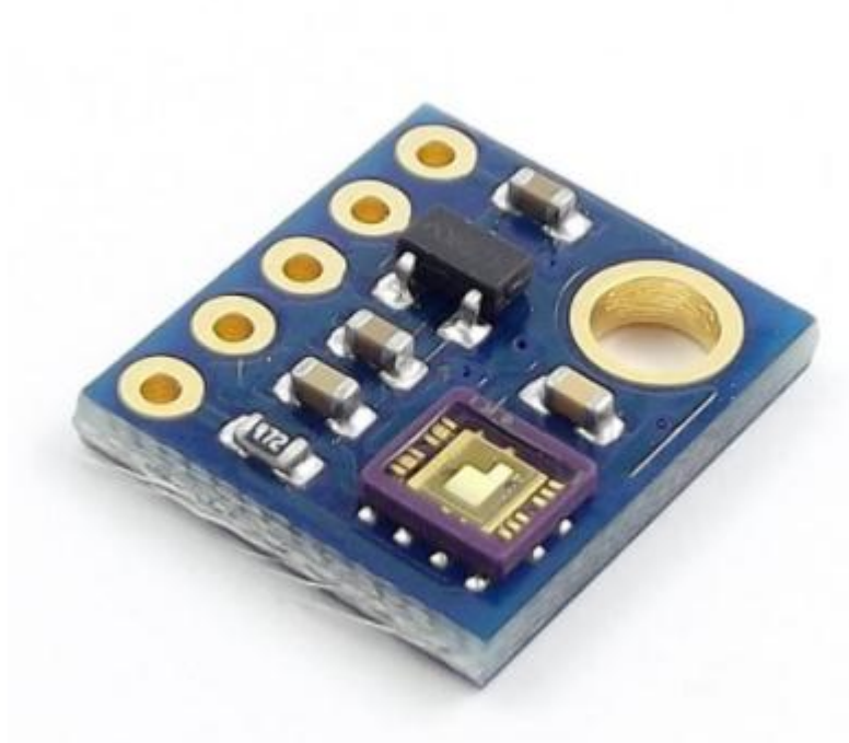
Figura 21 Sensor UV ML8511 Fuente: Naylamps Electronics, 2018
