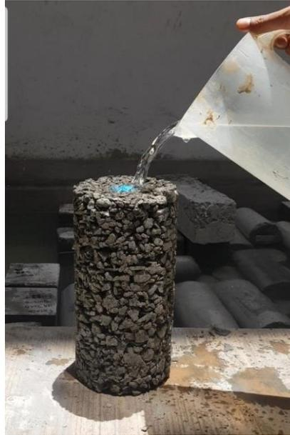
**Figura 24** Probeta permeable
