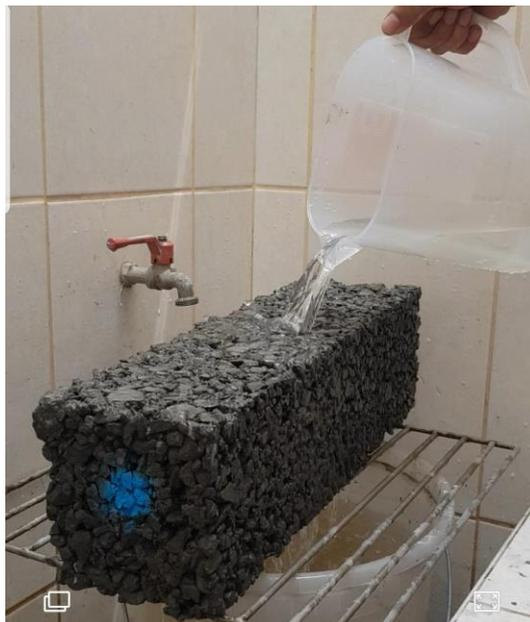
**Figura 35** viga permeable
