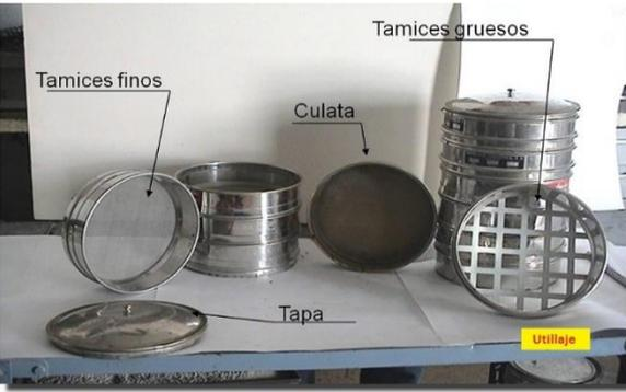
The image shows laboratory equipment for soil classification. It includes several sieves of different sizes, a funnel (Culata), a lid (Tapa), and a small yellow label that says 'Utilaje'. The sieves are arranged on a surface, and the funnel is placed on top of one of them.
