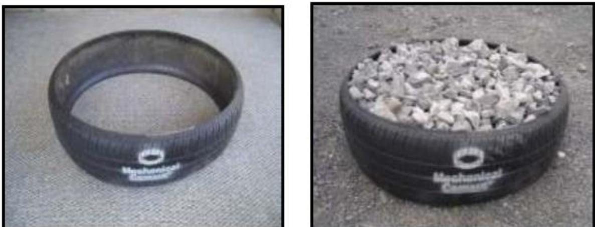
*Figura 3. Mechanical Cement® (izq.) y Mechanical Concrete® (dcha.)*
