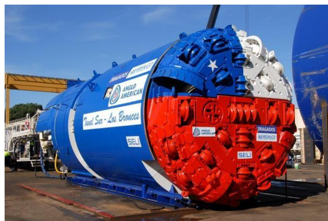
Figura 3. Tunnel Boring Machine
