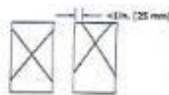
Type 1 Reasonably well formed cones on both ends, less than 1 in. (25 mm) of crushing through caps
