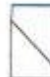
Type 4 Diagonal fracture with no cracking through ends; test with hammer to distinguish from Type 1
