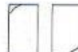
Type 5 Side fracture at top or bottom (occur commonly with unbraced cast)
