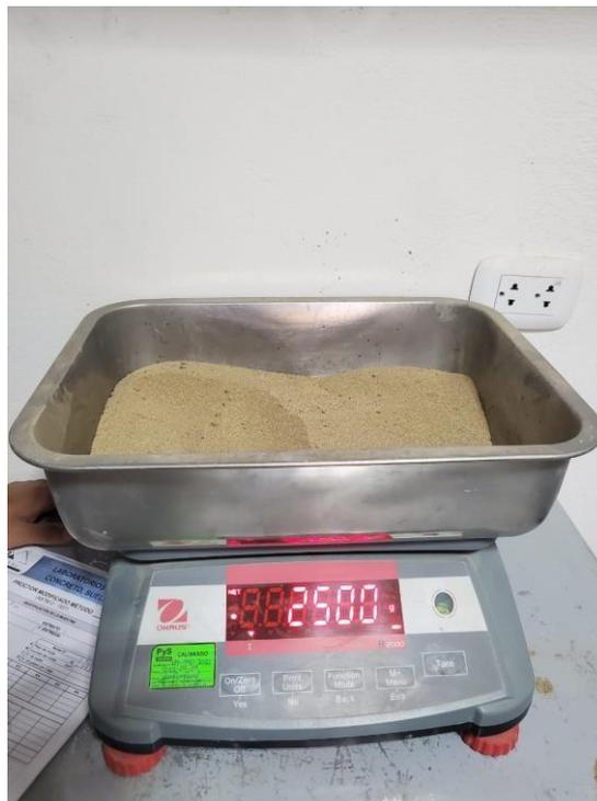
IMAGEN 14: TOMAMOS UNA MUESTRA DE 2.5KG PARA PROCEDER CON EL PROCTOR
