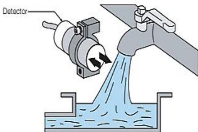
*Figura 14:* Detector de proximidad capacitivo, tomada de [https://download.schneider-electric.com/files?p\\_enDocType=Specification+guide&p\\_File\\_Name=600020K05-mtp-vol3.pdf&p\\_Doc\\_Ref=600020K05&\\_ga=2.106961410.105471583.1532975752-1044205147.1532975752](https://download.schneider-electric.com/files?p_enDocType=Specification+guide&p_File_Name=600020K05-mtp-vol3.pdf&p_Doc_Ref=600020K05&_ga=2.106961410.105471583.1532975752-1044205147.1532975752). Pág. 567.
