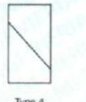
Type 4 Diagonal fracture with no cracking through ends; tap with hammer to distinguish from Type 1
