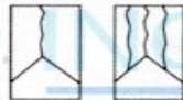
Type 2 Well-formed cone on one end, vertical cracks running through caps, no well-defined cone on other end
