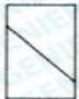
Type 4 Diagonal fracture with no cracking through ends; tap with hammer to distinguish from Type 1
