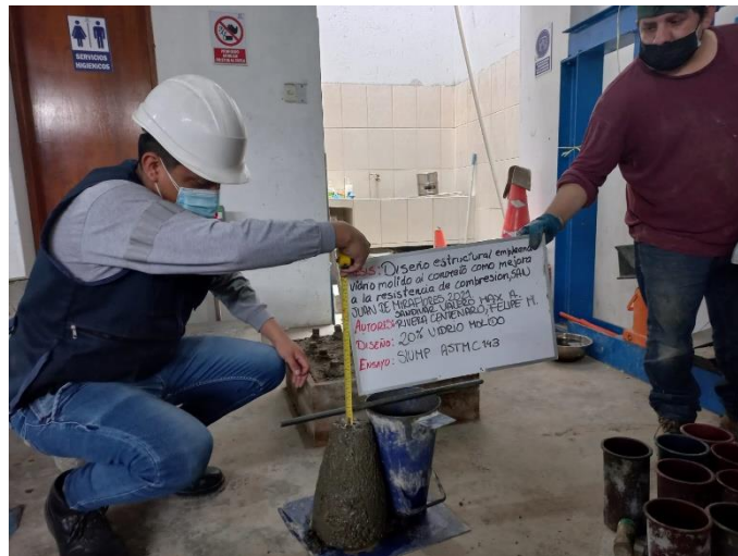
Figura 8. Ensayo Slump ASTM 143 – 20% V.M
