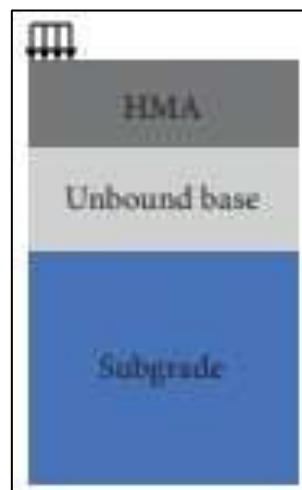
Figura 7. Estructura de un pavimento, tomado de «Mechanical properties of municipal solid waste incinerator (mswi) bottom ash as alternatives of subgrade materials», por Huang et al., 2020, p. 3
