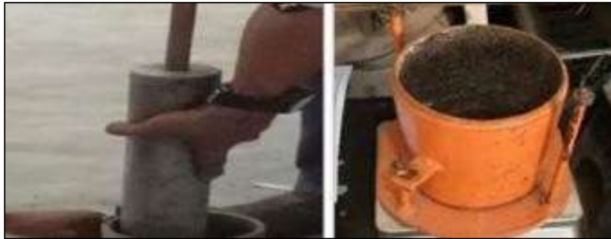
Figura 5. Compactación en laboratorio, tomado de «Analysis of soil compaction using proctor standards in highway construction design», por Mahardika et al., 2021, p. 4
