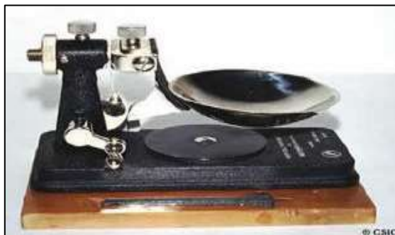
Figura 3. Cuchara de Casagrande, tomado de «Contribution to the knowledge of early geotechnics during the twentieth century : Arthur Casagrande», por Galindo, Lara y Guillán, 2018, p. 108
