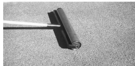
Fig. 8.8—Example of small roller used for compacting small paved area.
