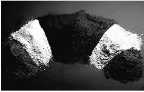
Fig. 12.2—Supplementary cementitious materials. From left to right: fly ash (Class C); metakaolin (calcined clay); silica fume; fly ash (Class F); slag; and calcined shale. (Reprinted with permission from Portland Cement Association.)
