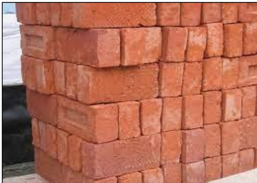
Figura 6: Ladrillo artesanal a base de arcilla cocida
