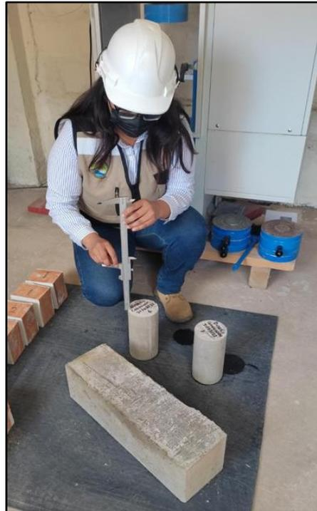
MEDICION Y PESAJE DEL CONCRETO – PROBETAS Y VIGAS
