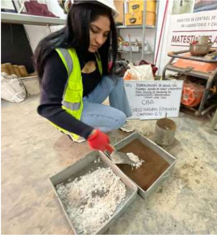
Ensayo de California Bearing Ratio
