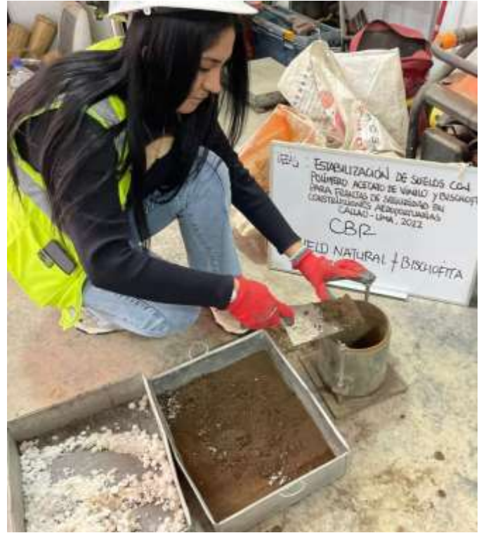
Ensayo de California Bearing Ratio
