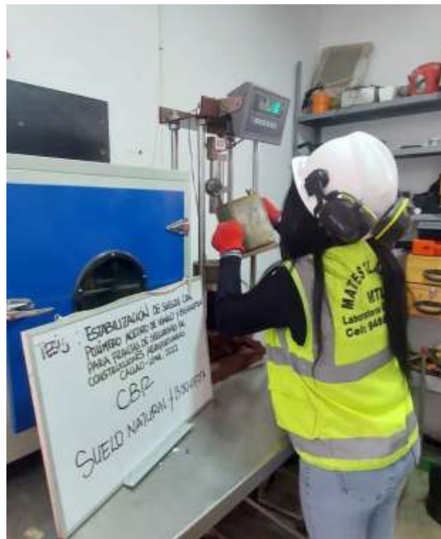
Ensayo de California Bearing Ratio
