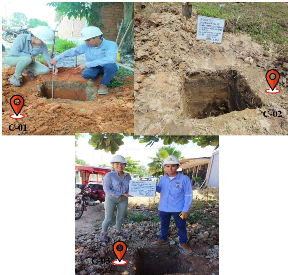
Figura 11. Calicatas in situ C-01, C-02, C-03
