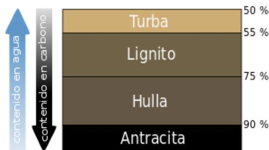
Figura 09. Principales tipos de carbón, Argonne National Laboratory.
