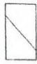
Type 4 Diagonal fracture with no cracking through ends; lap with hammer to distinguish from Type 1.
