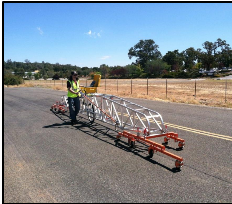
Figura 12. Perfilógrafo California (Surface Systems & Instruments, Inc.2017)
