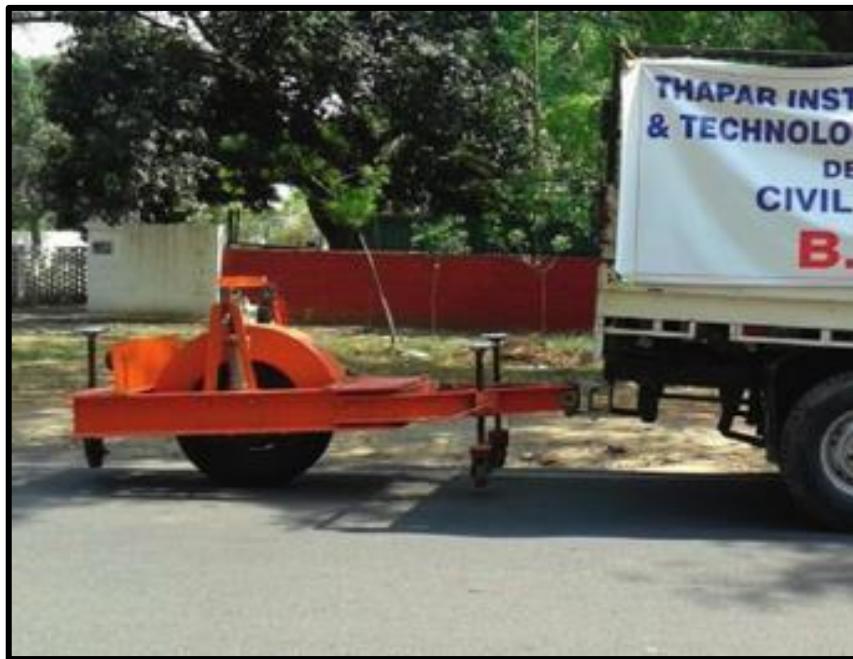
Figura 13. Bump Integrator (Chopra et al., 2018).
