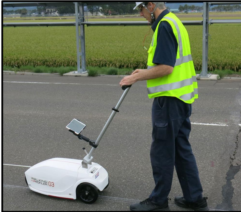
Figura 10. Walking Profiler (ARRB Systems 2023)
