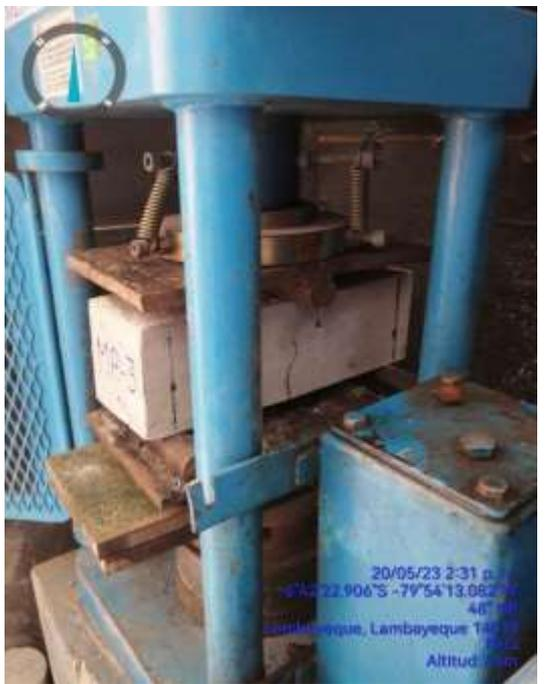
ROTURA MUESTRA EXPERIMENTAL - RESISTENCIA FLEXION 5% CS – 07 DIAS
