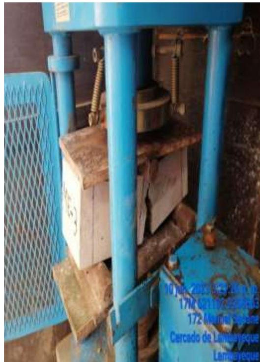
ROTURA MUESTRA EXPERIMENTAL - RESISTENCIA FLEXION 15% CS – 28 DIAS
