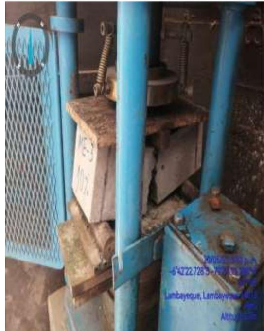
ROTURA MUESTRA EXPERIMENTAL - RESISTENCIA FLEXION 15% CS – 07 DIAS
