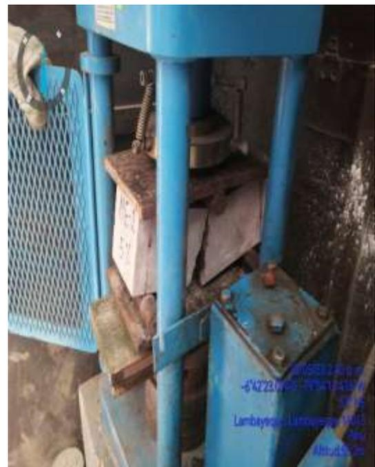
ROTURA MUESTRA EXPERIMENTAL - RESISTENCIA FLEXION 10% CS – 07 DIAS
