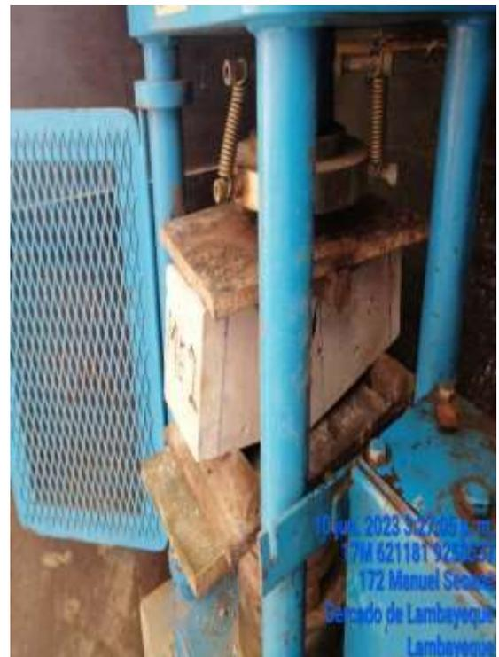
ROTURA MUESTRA EXPERIMENTAL - RESISTENCIA FLEXION 20% CS – 28 DIAS
