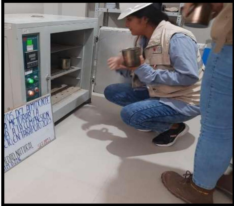
**IMAGEN 09: ENSAYO PESO ESPECIFICO- ASTM -C128**
