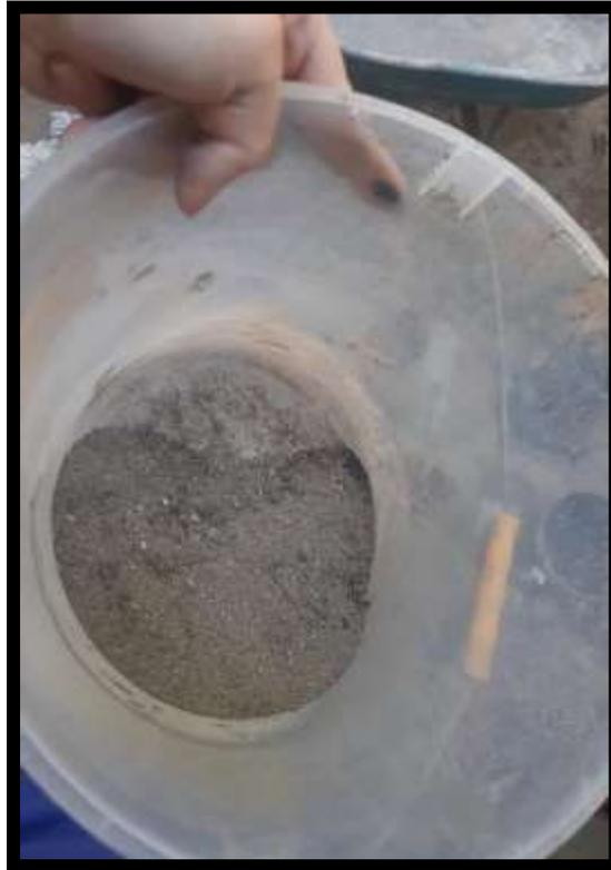
**IMAGEN 07: ENSAYO DE HUMEDAD NATURAL - NTP 339.185**
