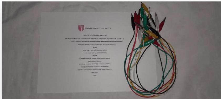
**Figura A.6: Cables cocodrilo**
