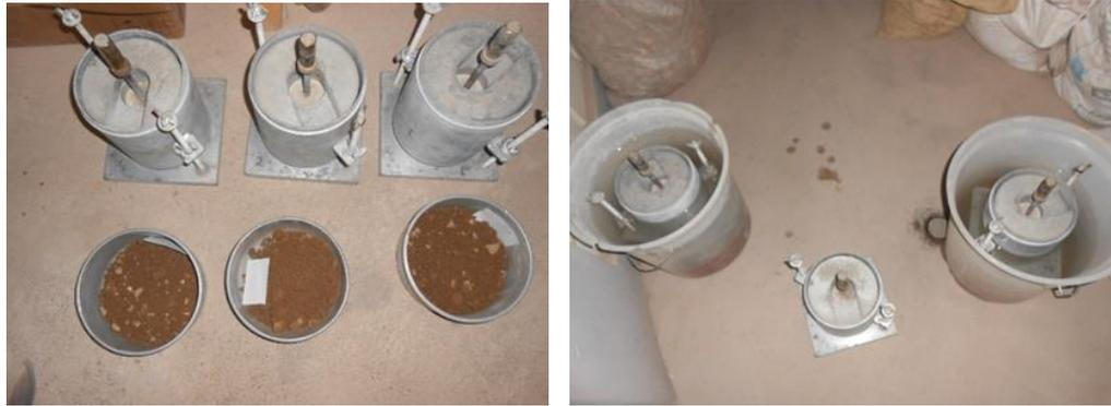
*Figura 8 Californian Bearing Ratio (CBR)*
