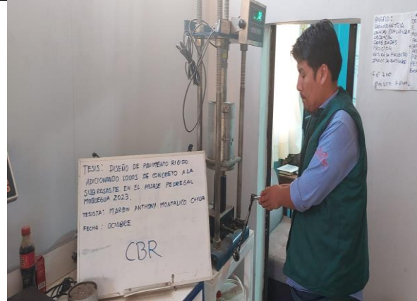
Figura 34. Ensayo de Californian Bearing Ratio (CBR)
