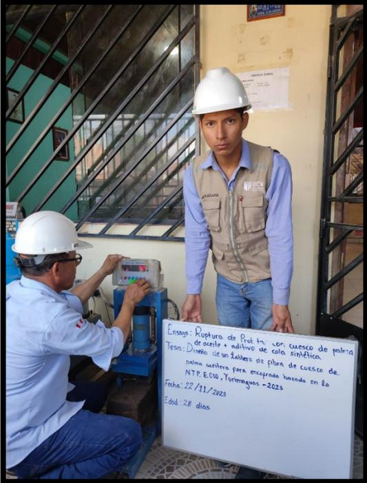
**IMAGEN 11. RUPTURA DE PROBETA EN COMPRESION**
