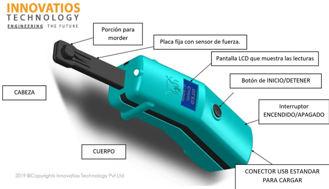
Figura 2. Partes del instrumento BYTE- Bite Force Measurement Device
