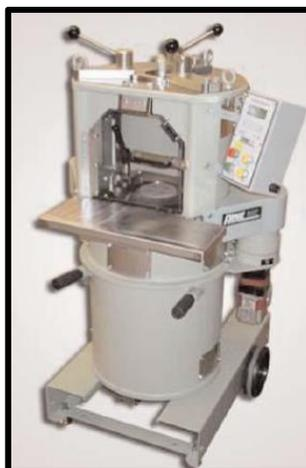
Figura 1. Superpave gyratory compactor (courtesy of Pine Equipment Company).
