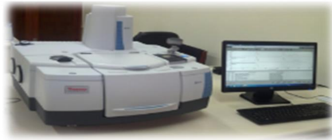
Figura 5: Thermo Fisher Nicolet iS50 FT-IR
