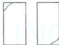
Type 5 Side fractures at top or bottom (occur commonly with unbanded caps)
