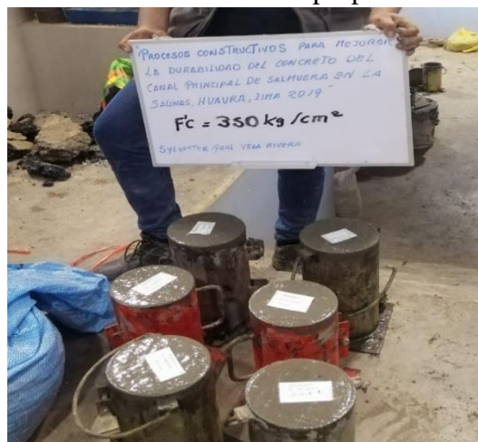
Figura 16: probetas elaboradas f'_c=350\text{kg/cm}^2
