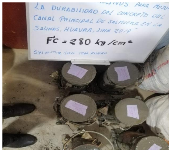
Figura 13: probetas elaboradas f'c=280\text{kg/cm}^2
