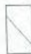
Type 4 Diagonal fracture with no crushing was observed; top and bottom to extrusion; more than Type 1
