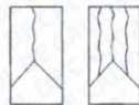
Type 2 Well-formed cone on one end, vertical cracks running through caps, no well-defined cone on other end
