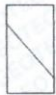
Type 4 Diagonal fracture with no cracking through ends; top with hammer to distinguish from Type 1
