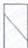
Type 4 Diagonal fracture with no cracking through ends; tap with hammer to distinguish from Type 1
