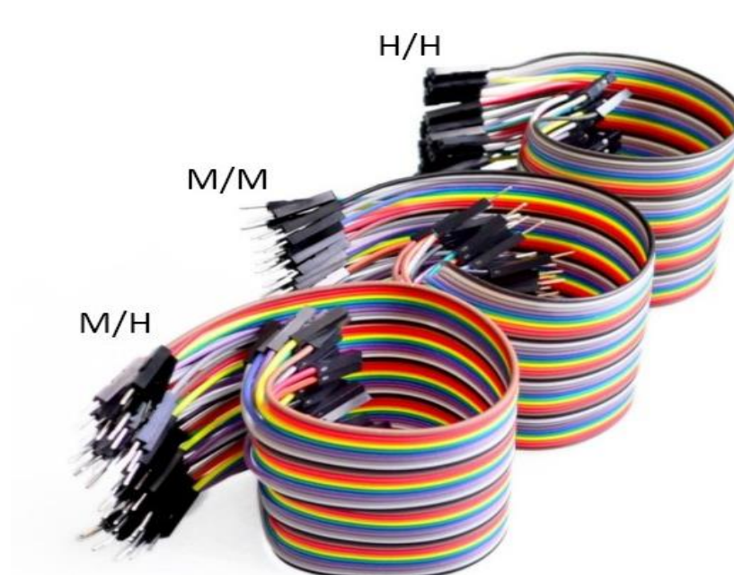
Figura 41. Cables jumper, dupont.
