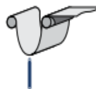
Break, tear & slack monitoring
