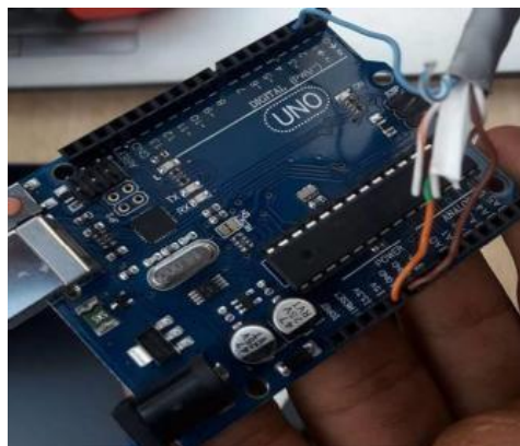
Fig. 15: Board Model UNO R3: Arduino 1
