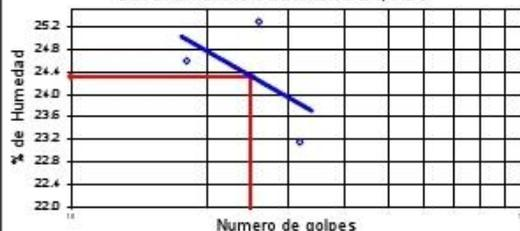
**D. ENSAYO DE LÍMITE PLÁSTICO E ÍNDICE PLÁSTICO (MTC E-111)**
