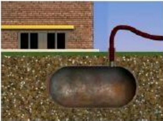
Fig. 7.6—Filling abandoned underground fuel- or oil-storage tank with cellular concrete (click on picture to view video).
