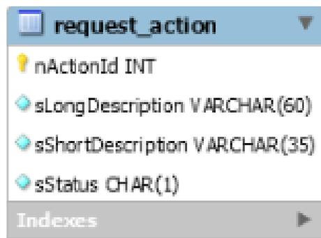
The screenshot displays the 'request\_action' table structure in SQL Server Enterprise Manager. The table contains the following columns:
