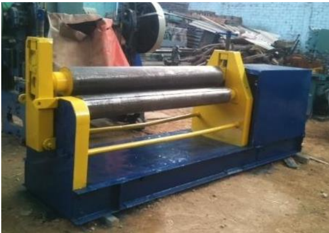
Figura 23: ROLA N°1. Potencia: 3.73KW, 3 \phi /380v/60Hz. Cant: 1
