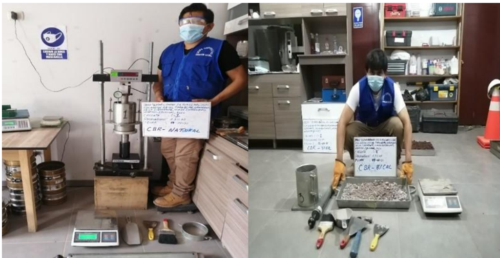
Figura 5. California Bearing Ratio (CBR) en laboratorio ASTM D-1883, MTC – E132
