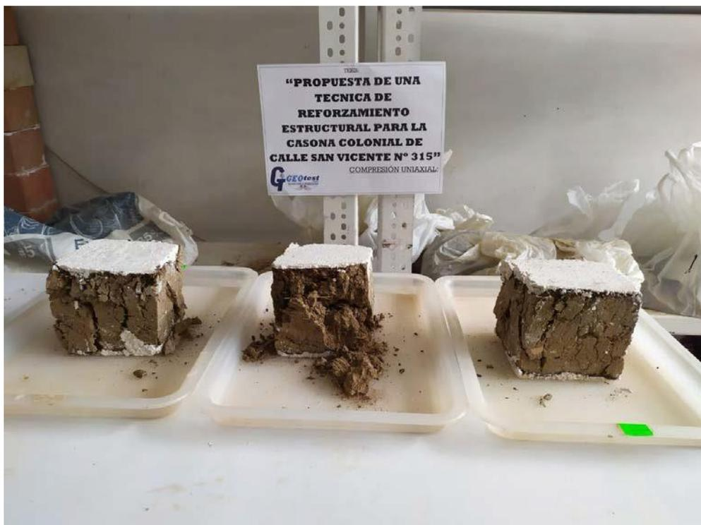
FIGURA-05 CUBOS PRISMATICO DESPUES DEL ENSAYO A COMPRESION
