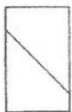
Type 4 Diagonal fracture with no cracking through ends, tap with hammer to distinguish from Type 1
