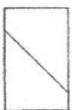
Type 4 Diagonal fracture with no cracking through ends, tap with hammer to distinguish from Type 1
